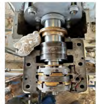
Replacement of Mechanical Seal for Brine Injection Pump BCP-213 by Site Maintenance
