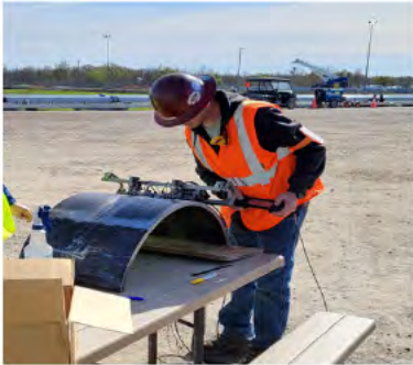
BC-LE-1759, Phased Array Weld Inspection Scanning Tool
