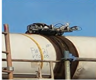
BC-LE-1759, Phased Array Weld Inspection Scanning Tool
